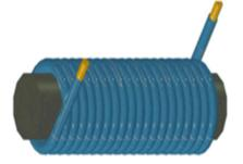
Figure 5 (a) Use of current to maintain the magnetic field
