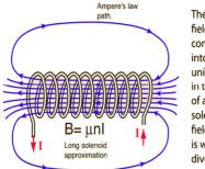
The magnetic field is concentrated into a nearly uniform field in the center of a long solenoid. The field outside is weak and divergent.
