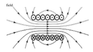
Figure 4. An electromagnet
